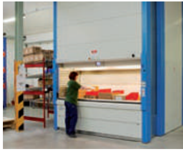
Kardex: automated high-capacity storage system.
