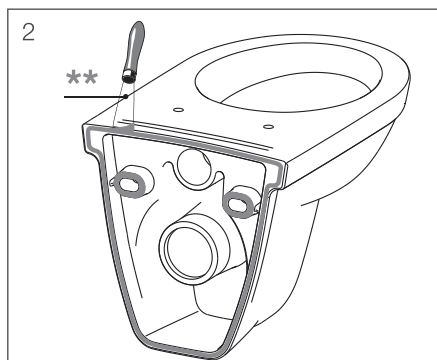
** Apply levelling paste layer of 5-10 mm.
